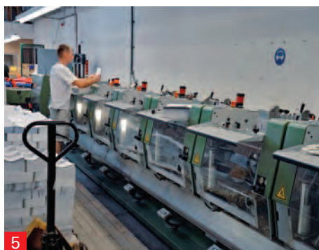
5 Digitally printed signatures, which are thread-sewn using the Ventura MC, are gathered using the BravoPlus saddle stitcher for larger runs.
